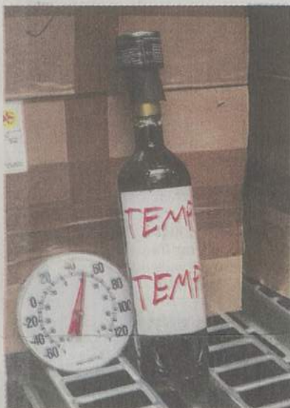
A test bottle is used to monitor temperature at Mana's climate-controlled storage facility in Jersey City.
